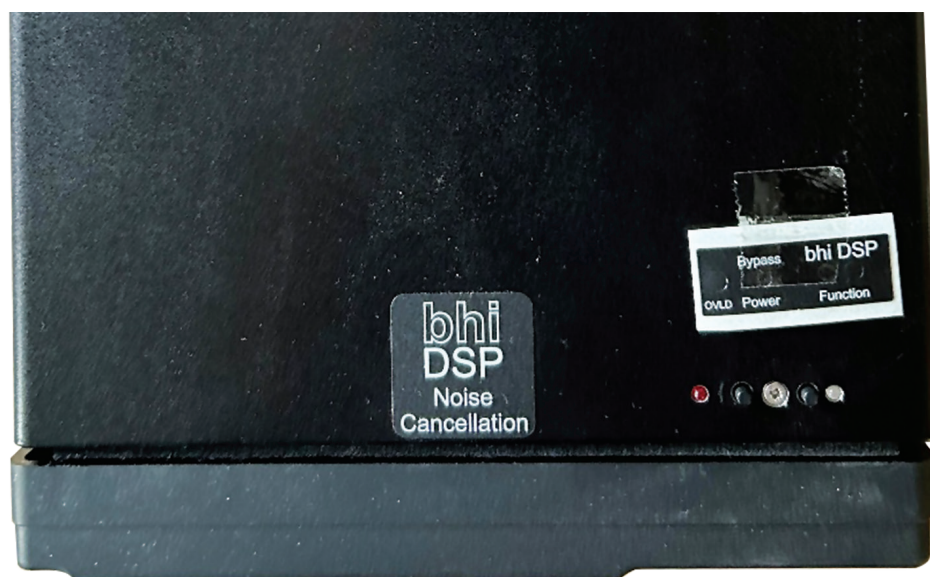
FIGURE 4: The keyboard switch assembly has been fitted to the outer casing of the speaker.
